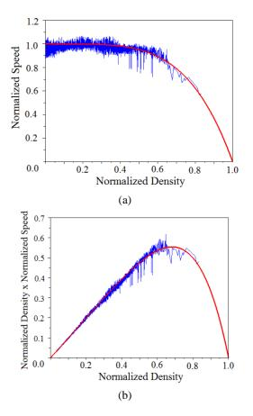
Fig 2: (a) The normalized density-normalized speed and (b) a representation of normalized density vs traffic flow behavior. The blue curve shows the actual data derived from the real-time traffic data, the approximated model is represented by the red curve.
