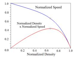
Fig 1: represents the normalized speed vs normalized density and the flow vs normalized density using the proposed power law model using m=0.6 ans n=5. The marked point represents the critical point where flow is at maximum.
